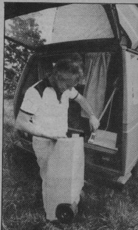
Novel idea in motor caravan is a detachable water tank on own little wheels. Water fed from it by immersed pur
