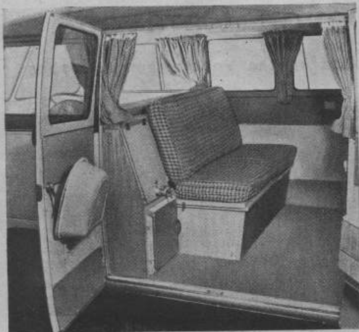
Wide double nearside doors open on the interior, which has two wide facing bench seats (a table can be clipped between them), a water tank above a cold-store food cabinet, and a hinged washbasin on the forward door.
