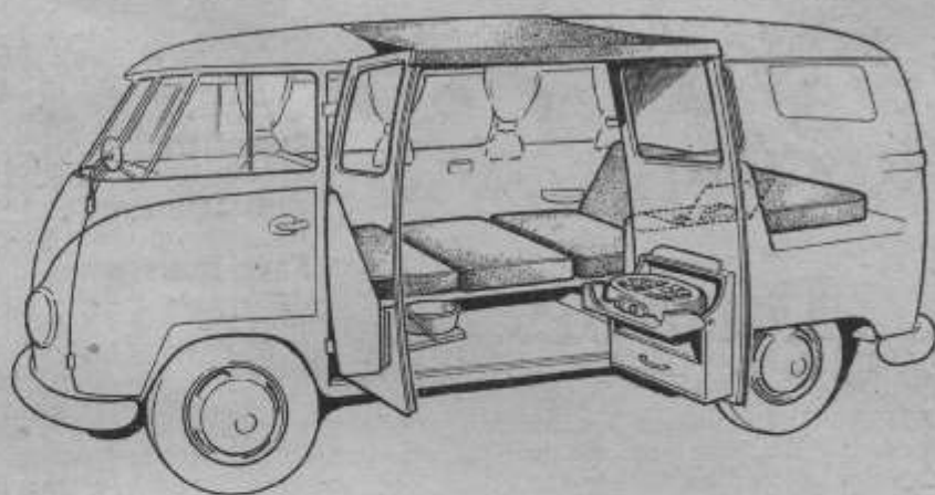
As arranged for sleeping, the seats make up into a double bed supported by the table in the centre. There is a single bunk for a child at the rear and a second child could be accommodated on the driving seat.
